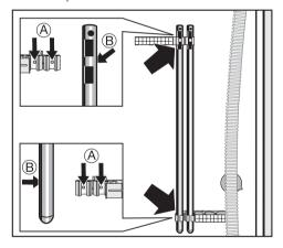
Secure the transit bars to the back of the washing machine. Make sure that holes (B) are fitted over retainers (A). The washing machine must not be moved without the transit bars in place.
